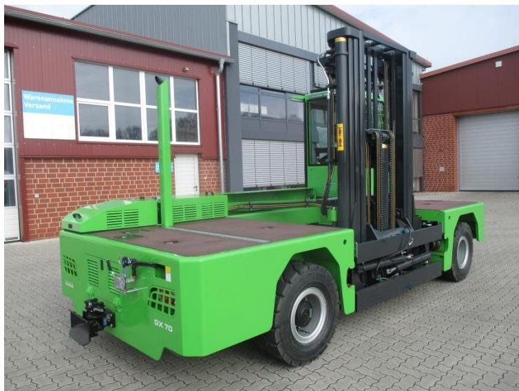
*Duo-Matic quick couplers at front and rear allow for quick and safe coupling.*
